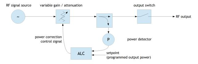
The ALC loop and the output blanking switch are both depicted in *Figure 1*.
